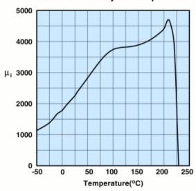
Measured on an 18/10/6mm toroid at 100kHz.
