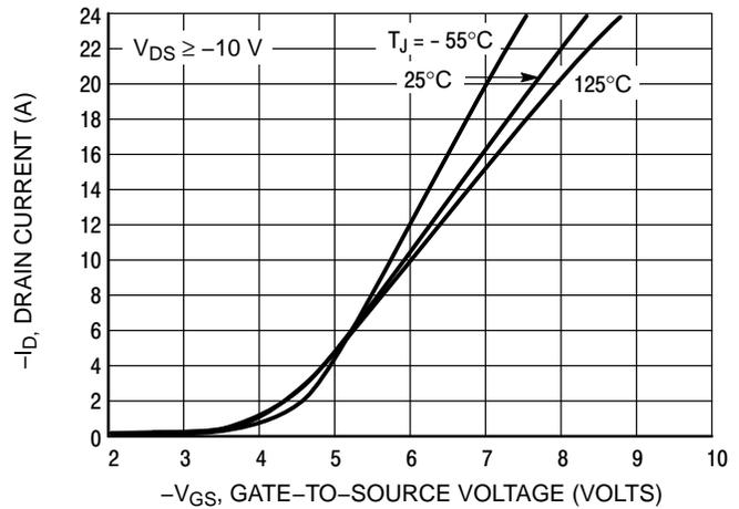
Figure 2. Transfer Characteristics
