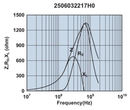
Impedance, reactance, and resistance vs. frequency.
