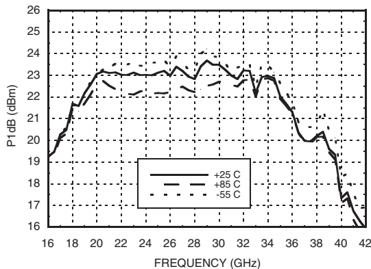
P1dB vs. Temperature
