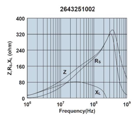
Impedance, reactance, and resistance vs. frequency.
