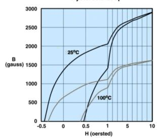
Measured on a 17/10/6mm toroid at 10kHz.
