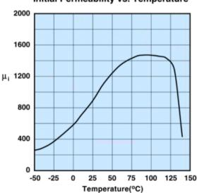
Measured on a 17/10/6mm toroid at 100kHz.
