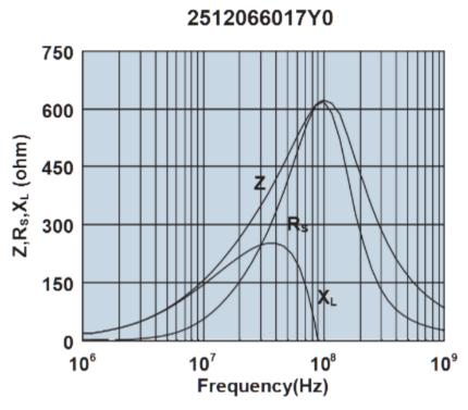
Impedance, reactance, and resistance vs. frequency.
