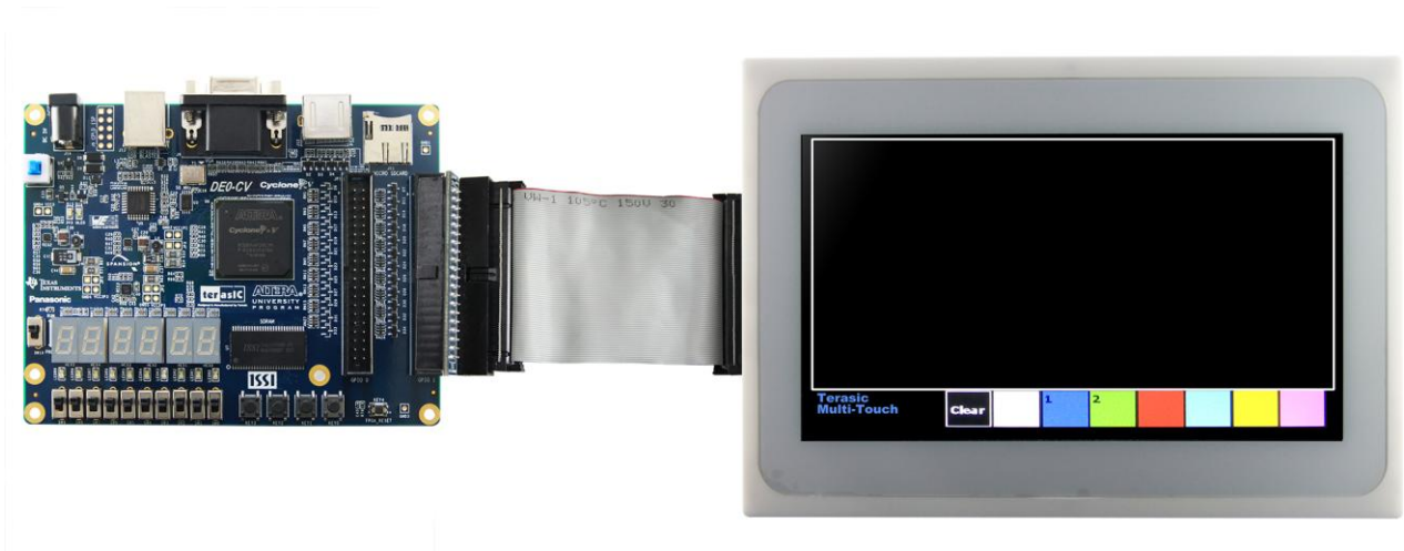
Figure 5-7 Hardware Setup with DE0-CV
