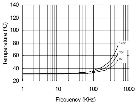
Figure 32. IR2106S vs. Frequency (IRFBC20),
