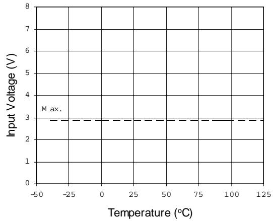
Figure 8A. Logic "1" Input Voltage
