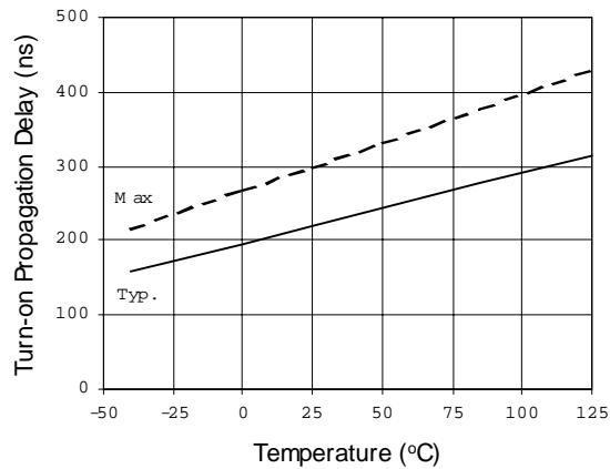
Figure 4A. Turn-on Propagation Delay
