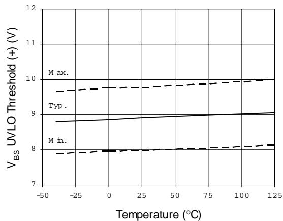
**Figure 19.  $V_{BS}$  Undervoltage Threshold (+)
