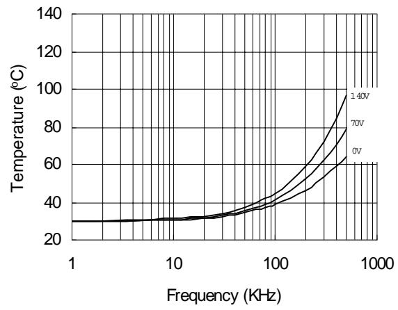
**Figure 38. IR21064S vs. Frequency (IRFBC40),**
