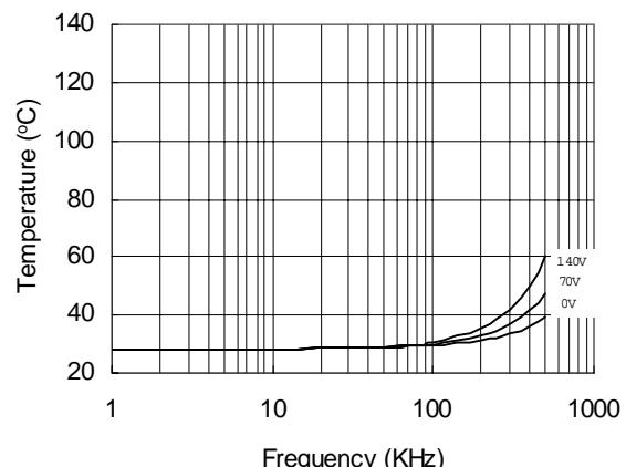
Figure 36. IR21064S vs. Frequency (IRFBC20),
