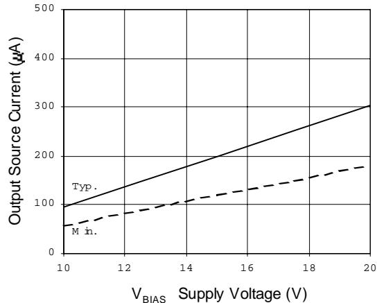
**Figure 21B. Output Source Current
