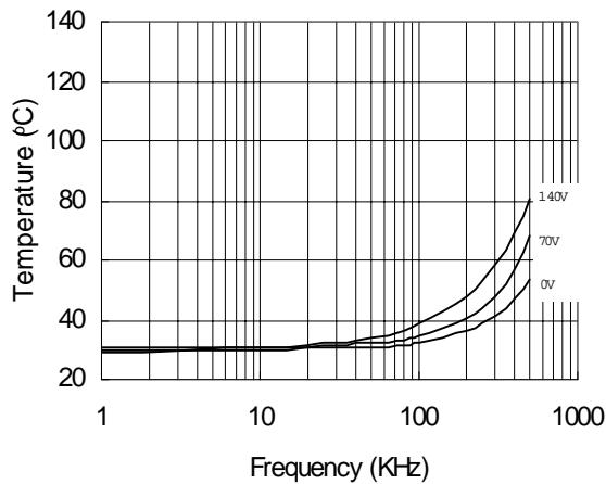
**Figure 37. IR21064S vs. Frequency (IRFBC30),**
