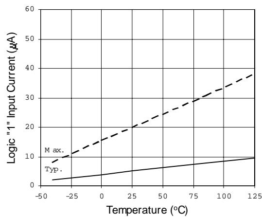
Figure 15A. Logic "1" Input Current vs. Temperature
