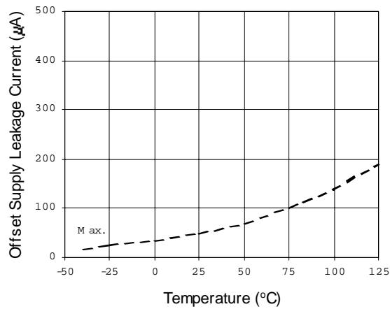
Figure 12A. Offset Supply Leakage Current vs. Temperature
