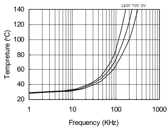
Figure 35. IR2106S vs. Frequency
