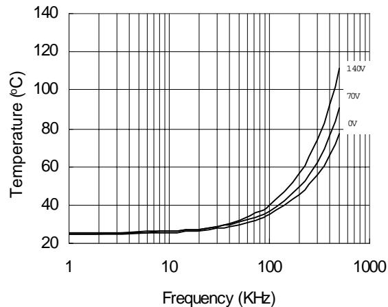
Figure 33. IR2106S vs. Frequency (IRFBC30),
