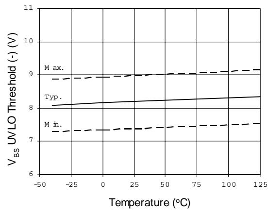
**Figure 20.  $V_{BS}$  Undervoltage Threshold (-)
