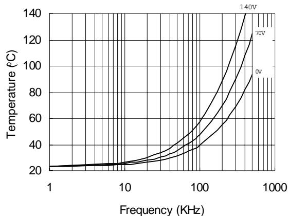
Figure 31. IR21064 vs. Frequency (IRFPE50),
