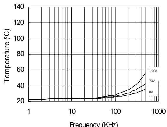
**Figure 28. IR21064 vs. Frequency (IRFBC20),**
