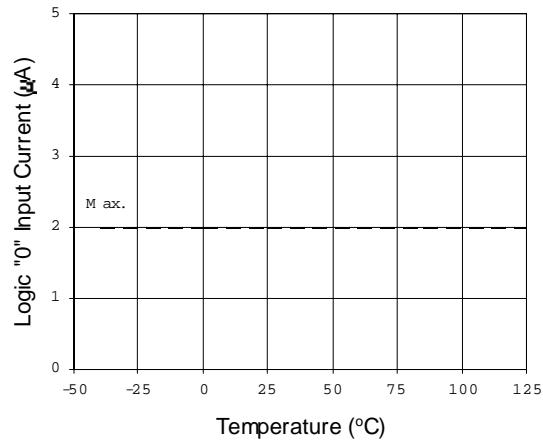
Figure 16A. Logic "0" Input Current vs. Temperature
