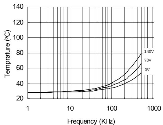
Figure 24. IR2106 vs. Frequency (IRFBC20),
