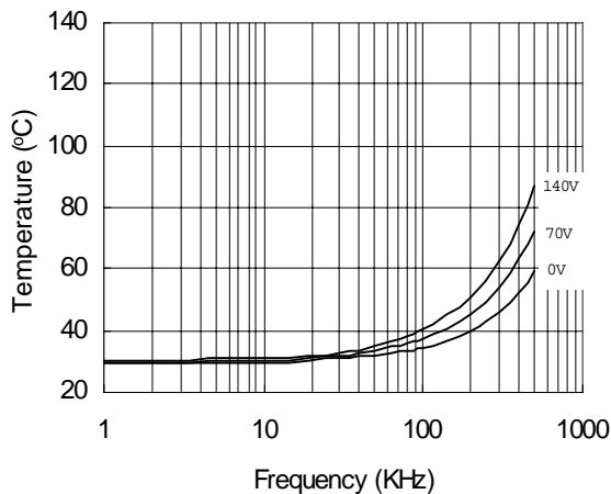
**Figure 25. IR2106 vs. Frequency (IRFBC30),**
