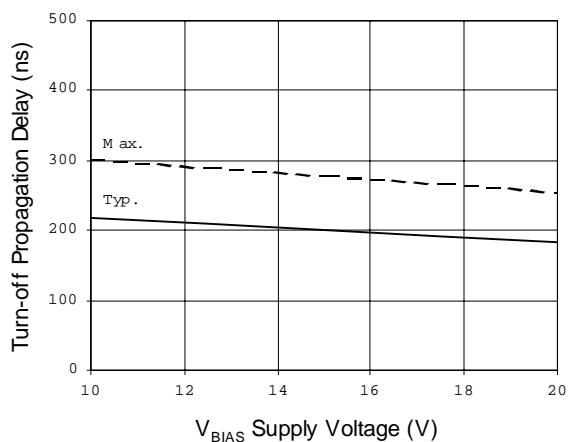
Figure 5B. Turn-off Propagation Delay
