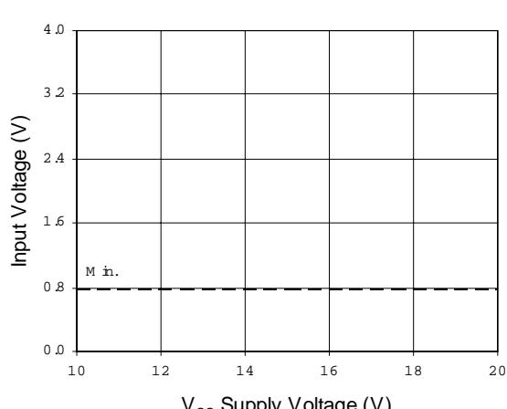
Figure 9B. Logic "0" Input Voltage
