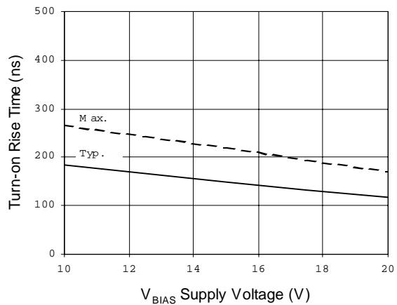
**Figure 6B. Turn-on Rise Time vs. Supply Voltage**
