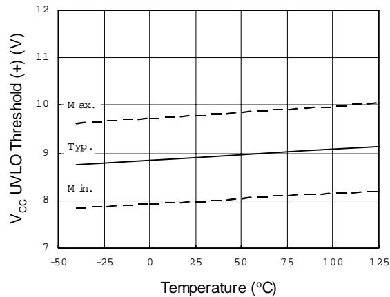
Figure 17.  $V_{\text{CC}}$  Undervoltage Threshold (+) vs. Temperature
