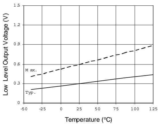
Figure 11A. Low Level Output Voltage vs. Temperature
