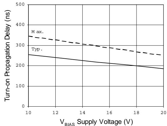
Figure 4B. Turn-on Propagation Delay
