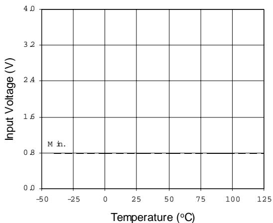
Figure 9A. Logic "0" Input Voltage
