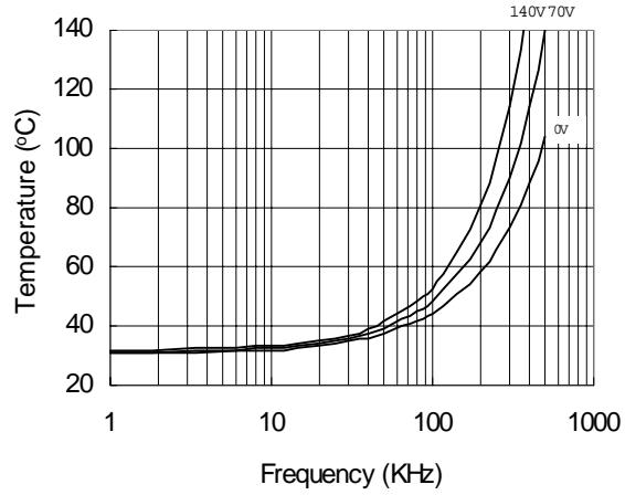
Figure 34. IR2106S vs. Frequency (IRFBC40),
