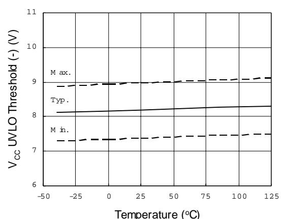
Figure 18.  $V_{\text{CC}}$  Undervoltage Threshold (-) vs. Temperature
