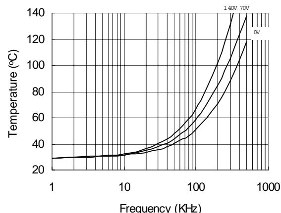
**Figure 27. IR2106 vs. Frequency (IRFPE50),**
