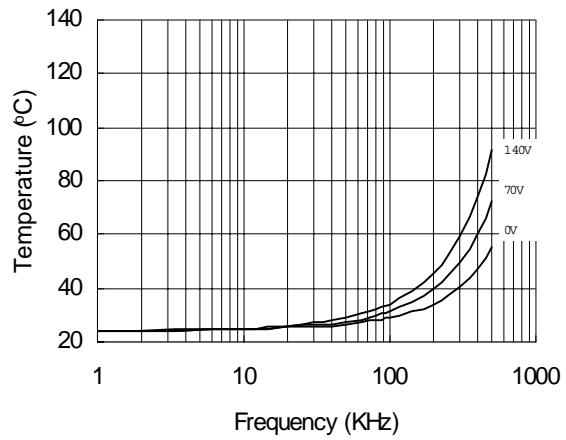
Figure 30. IR21064 vs. Frequency (IRFBC40),
