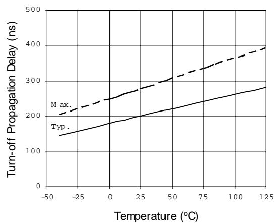
Figure 5A. Turn-off Propagation Delay
