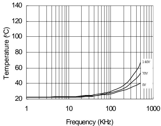
Figure 29. IR21064 vs. Frequency (IRFBC30),
