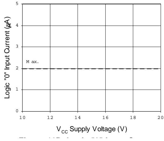
Figure 16B. Logic "0" Input Current vs. Supply Voltage
