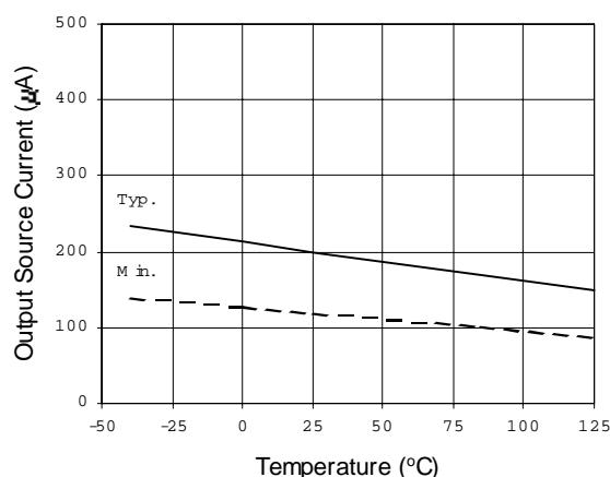
**Figure 21A. Output Source Current
