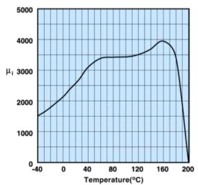
Measured on a 17/10/6mm toroid at 10kHz.
