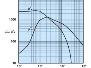
Measured on a 2673000301 bead using the HP 4284A and the HP 4291A.
