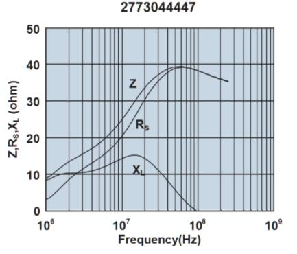
Impedance, reactance, and resistance vs. frequency.
