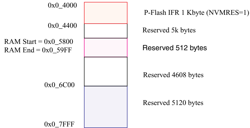
Figure 17-2. Memory Controller Resource Memory Map (NVMRES=1)
