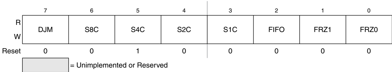
Figure 8-6. ATD Control Register 3 (ATDCTL3)
