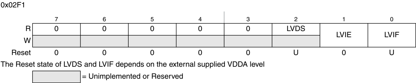
Figure 4-18. Low Voltage Control Register (CPMULVCTL)
