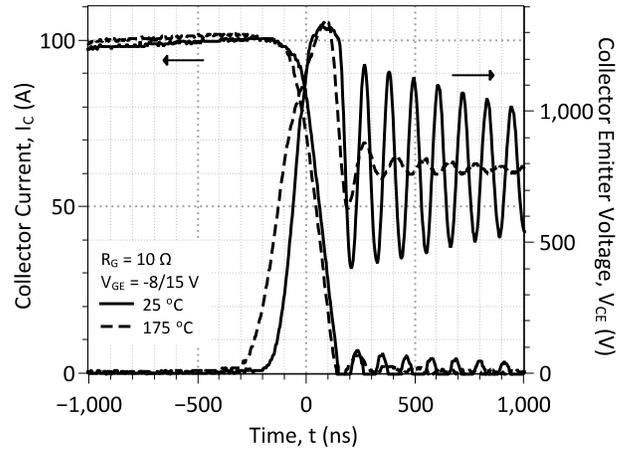
**Figure 8: Typical Hard-Switched IGBT Turn Off Waveforms**
