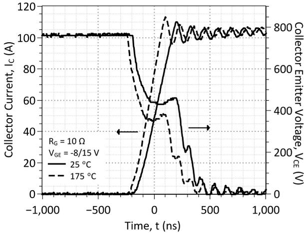
**Figure 7: Typical Hard-Switched IGBT Turn On Waveforms**
