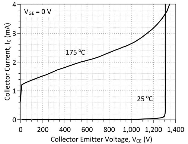
**Figure 4: Typical Blocking Characteristics**
