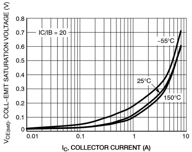
Figure 9. MJD45H11 Saturation Voltage
