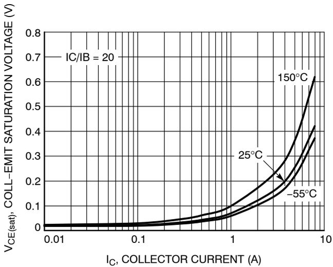
Figure 8. MJD44H11 Saturation Voltage
