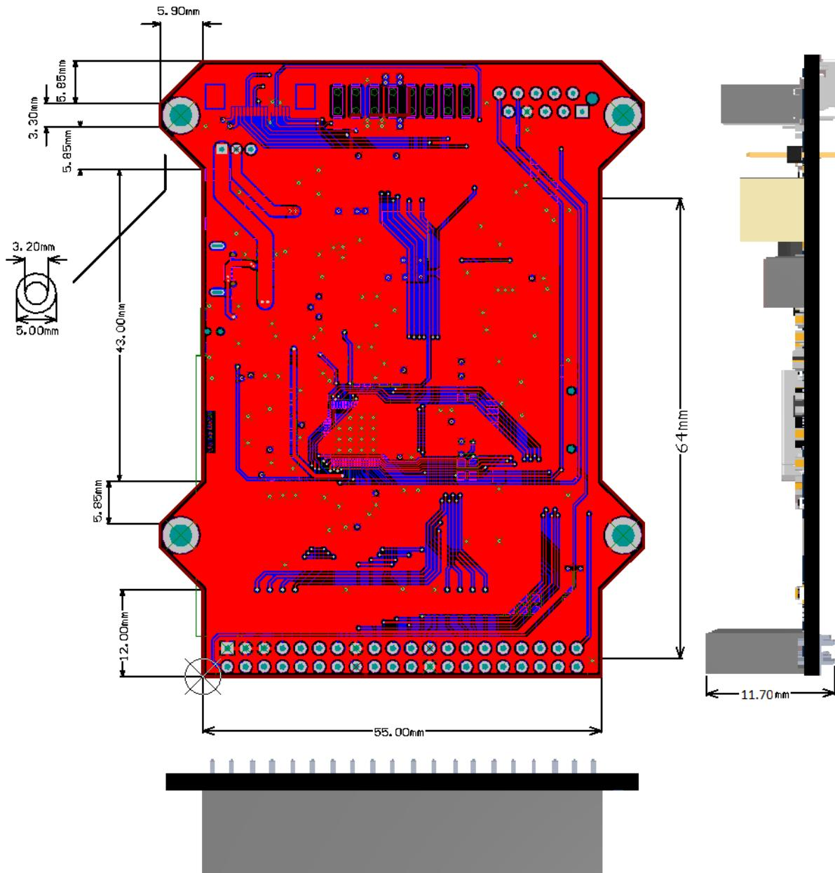
Figure 6-1 – MM930Lite PCB Dimensions
