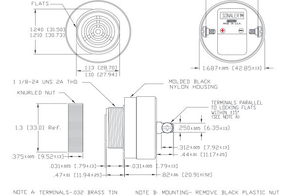
PLATED, TAPPED FOR #6-32 SCREW. TWO #6-32 NICKEL
