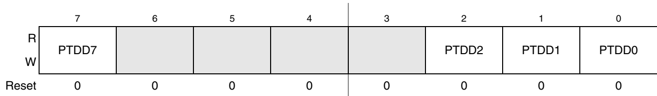
Figure 6-17. Port D Data Register (PTDD)
