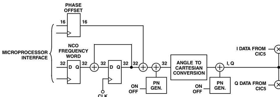
Figure 33. Numerically Controlled Oscillator and QAM Mixer
