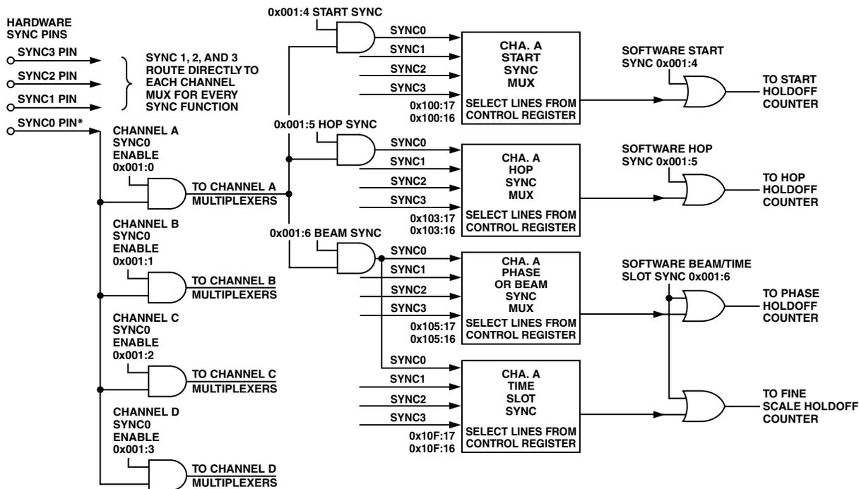
\*HARDWARE SYNC 0 IS CONFIGURED TO MATCH THE SYNC FUNCTION OF THE AD6622 FOR PIN COMPATIBILITY
