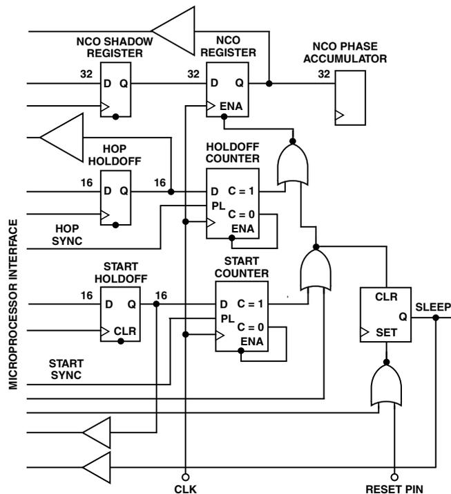
Figure 36. NCO Shadow Register and Hold-Off Counter
