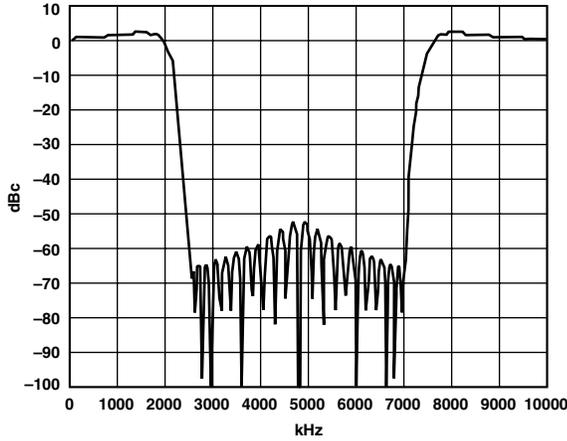
Figure 43. RAM Coefficient Filter, Frequency Response for WBCDMA
