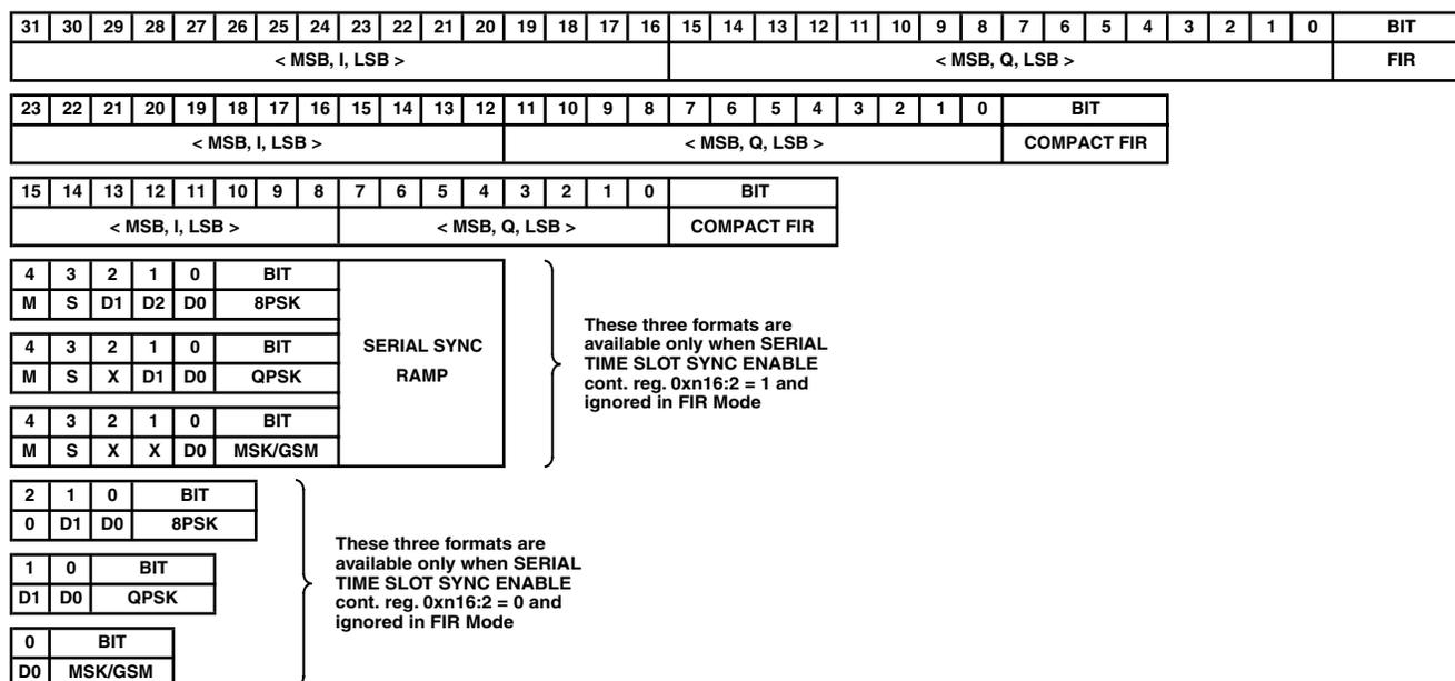
M = mode bit. If M = 0, then the MSB of 3-bit mode select word at 0xn0C:6 is set to 0 (this is also called MODE 0). If M = 1, then the MSB is set to 1 and this is MODE 1. Mode allows quick format changes via the serial port, for example, 010 = GMSK and 110 = 3pi/8PSK. The value m should be held for the duration of the time slot since the value of m will only be updated after the RCF Scale Holdoff Counter reaches a value of 1 (see below).
