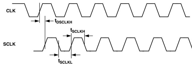
Figure 5. SCLK Switching Characteristics (Divide by 1)
