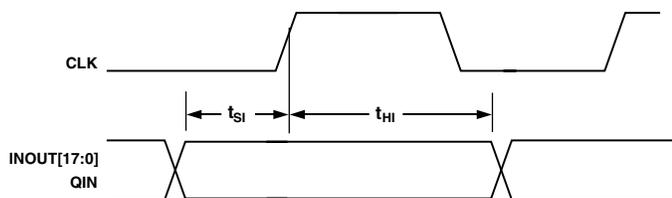
Figure 2. Wideband Input Timing
