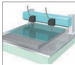
Ideal for measuring glass thickness and nozzle gaps when coating glass with resist or sealer.
