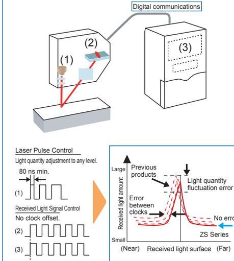
High-speed digital communications (LVDS) used between Sensor and Controller. Image signal stabilizes because the clock error between the control signal from the Controller and the light reception device disappears. Optimum light quantity adjustment is possible with laser power algorithms that can be adjusted to any level, which facilitates super high resolution.
