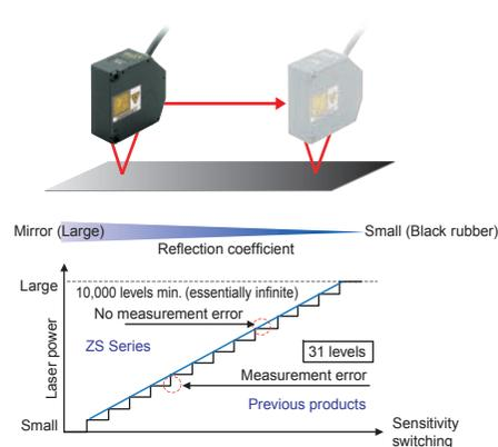
Light quantity adjustment algorithms have evolved for stable measurement of a variety of measurement objects. Even if the workpiece status changes suddenly, the sensitivity can compensate at any level so there is no measurement error from sensitivity switching.
