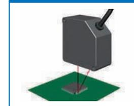
Measuring Shape for Positioning Laminated Ceramics
