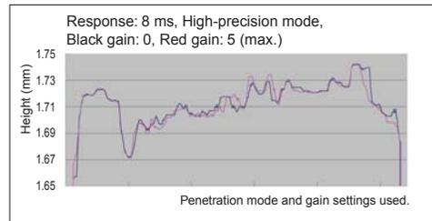
PCB shapes can be measured without burs or waveform disruptions.
