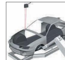
Protruding objects and steps can be measured from a distance for measurement objects that cannot be accessed easily.
