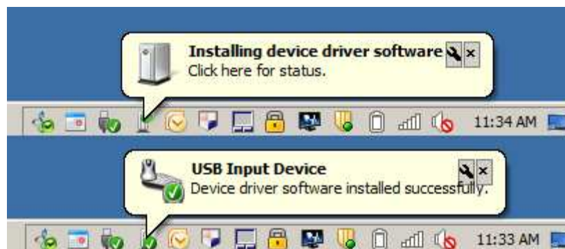
Figure 5. Typical Response After Connecting OPT3001EVM to the Computer
