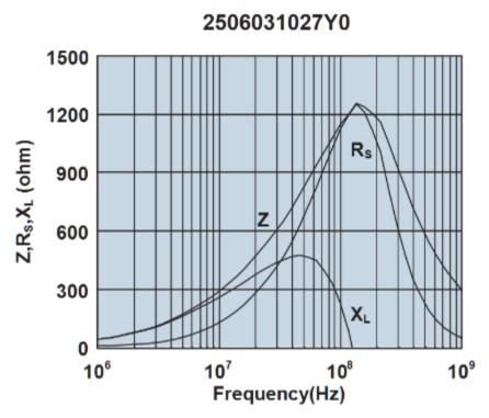
Impedance, reactance, and resistance vs. frequency.
