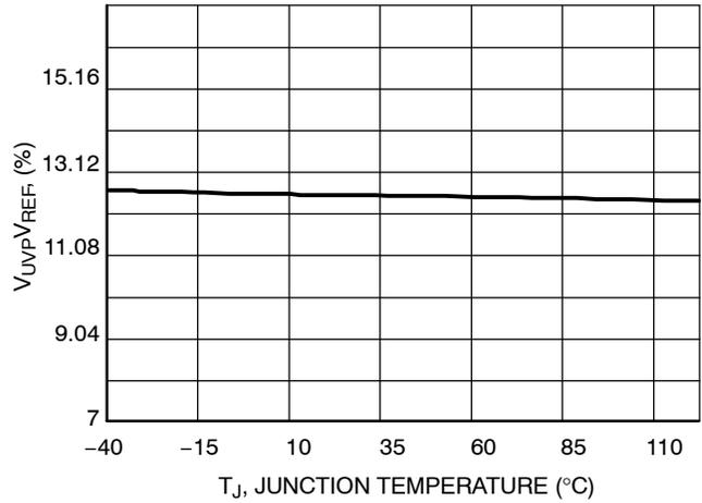
**Figure 8. Ratio (V<sub>UVP</sub>/V<sub>REF</sub>) vs. Temperature**
