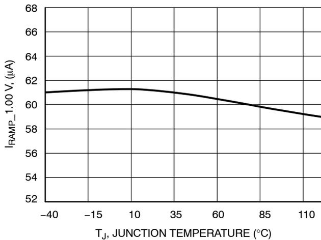
**Figure 40. Pin 7 Source Current @ V<sub>PIN4</sub> = 1.0 V vs. Temperature**
