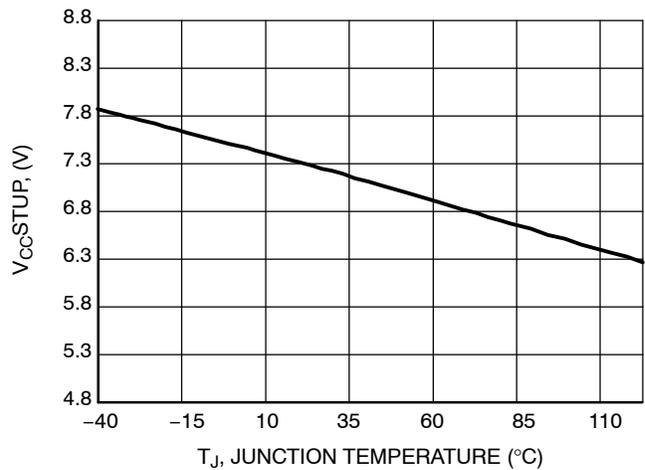
**Figure 12. V<sub>CC</sub> Threshold Below which the Startup Current Source Turns on vs. Temperature**
