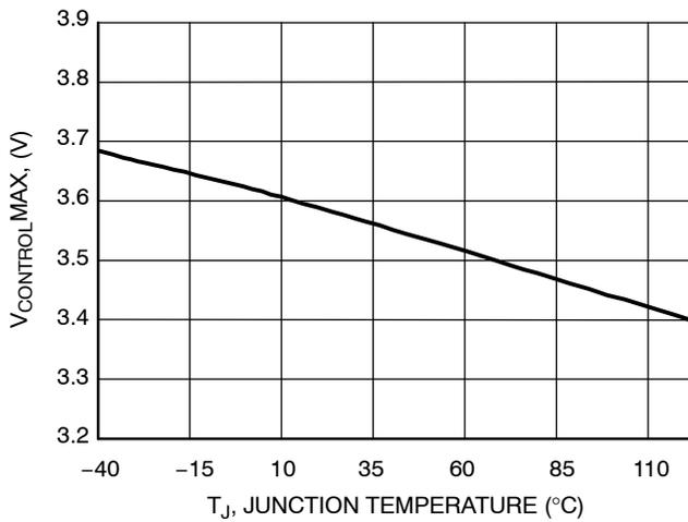
**Figure 23. V<sub>CONTROL</sub> Maximum Voltage vs. Temperature**
