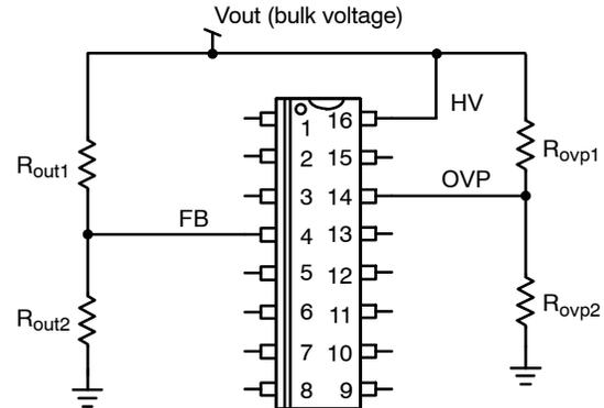
Figure 62. Configuration with Two Separate Feedback Networks
