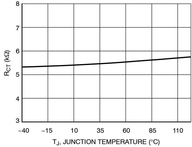
**Figure 43. Ratio Pin 7 Clamp Voltage / (Pin 7 Charge Current) that is (V<sub>CLCRM</sub> / I<sub>RAMP</sub>) @ V<sub>PIN6</sub> = 0 V and V<sub>PIN4</sub> = 1.75 V**
