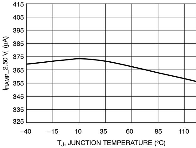
**Figure 42. Pin 7 Source Current @ V<sub>PIN4</sub> = 2.5 V vs. Temperature**
