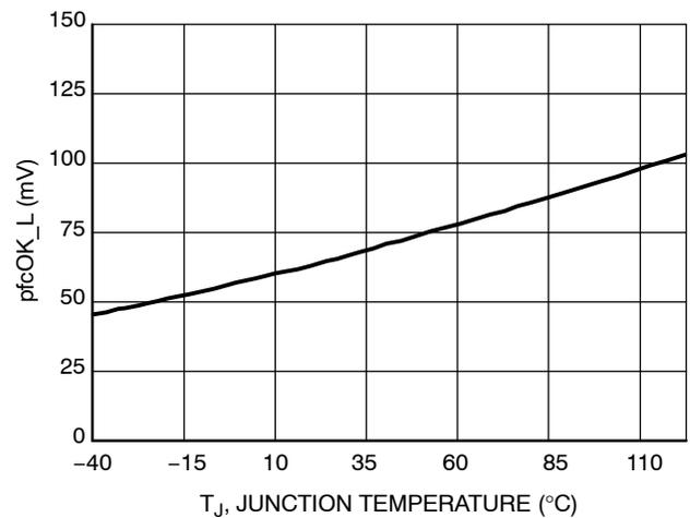
**Figure 30. pfcOK Pin Low Level Voltage vs. Temperature**
