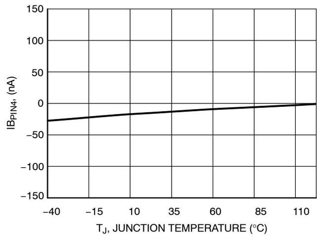
**Figure 22. Feedback Pin Bias Current vs. Temperature (@ V<sub>pin4</sub> = V<sub>REF</sub>)**
