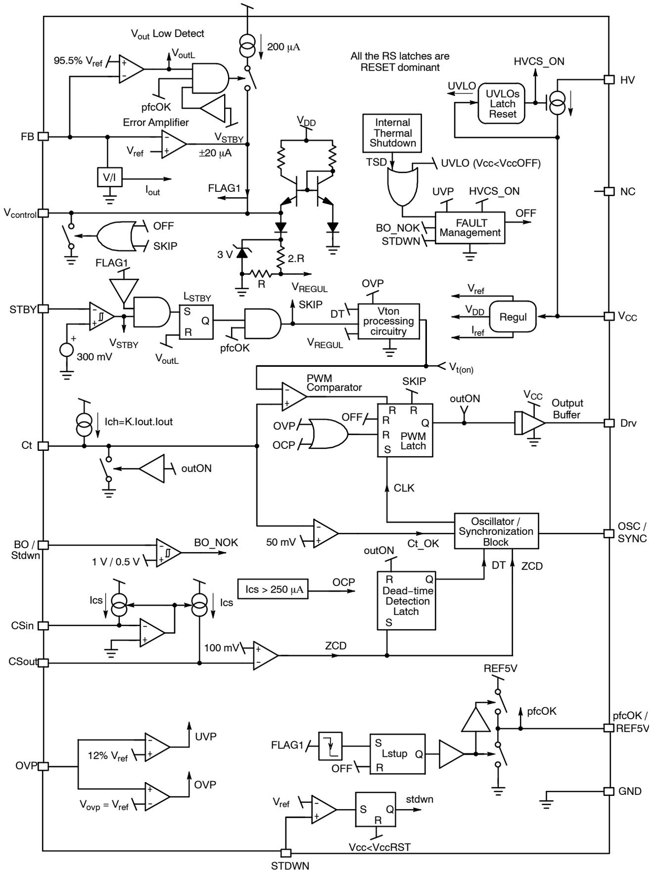
Figure 51. Block Diagram
