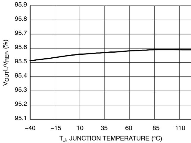
**Figure 25. Ratio (V<sub>OUT</sub> Low Detect Threshold) / V<sub>REF</sub> vs. Temperature**
