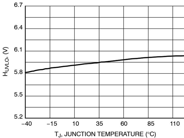
**Figure 11. Difference (V<sub>CC\_ON</sub> - V<sub>CC\_OFF</sub>) vs. Temperature - NCP1605/B**
