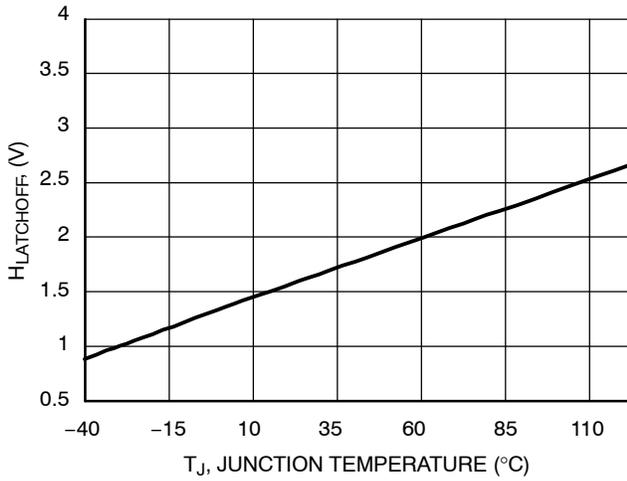
**Figure 13. Difference ( $V_{CCOFF} - V_{CCSTUP}$ ) vs. Temperature**
