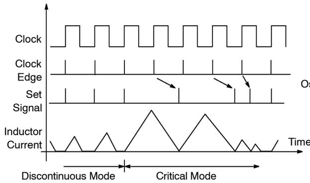
**Figure 65. Oscillator Timing Diagram**
