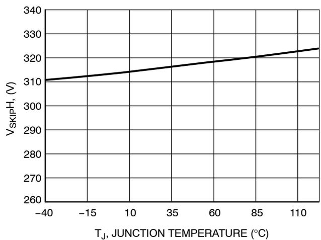
**Figure 47. Skip Cycle Threshold (V<sub>PIN1</sub> Falling) vs. Temperature**
