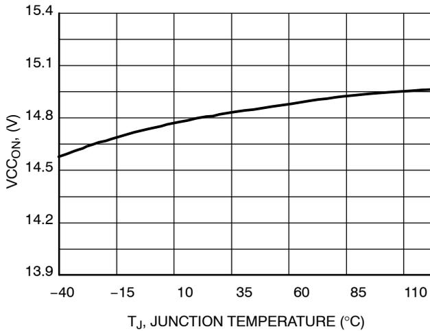
**Figure 9. V<sub>CC</sub> Turn on Threshold vs. Temperature (V<sub>CC</sub> Raising Up) - NCP1605/B**
