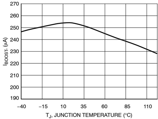
**Figure 26. Pin 3 Source Current when (V<sub>OUT</sub> Low Detect Threshold) is Activated vs. Temperature**
