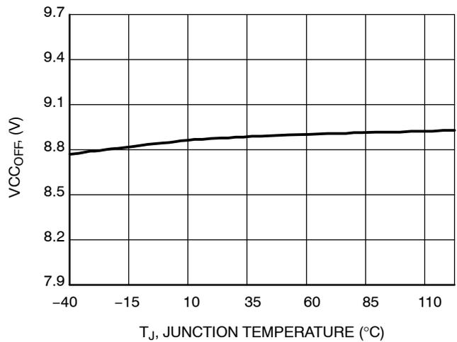
**Figure 10. V<sub>CC</sub> Minimum Operating Voltage After Turn On - NCP1605/B**
