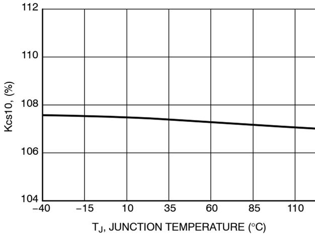
**Figure 44. Ratio (I<sub>PIN6</sub> / I<sub>PIN5</sub>) @ I<sub>PIN5</sub> = 10 µA vs. Temperature**
