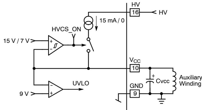
(When high, "UVLO" indicates that the circuit is not properly fed and it sets the Fault latch to turn off the circuit)
