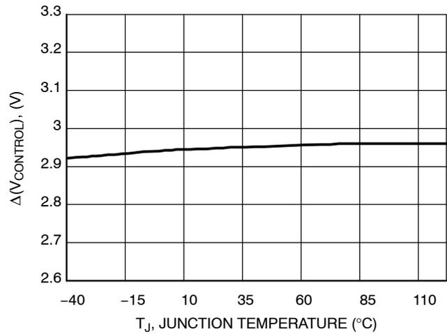
**Figure 24. V<sub>CONTROL</sub> Maximum Swing (ΔV<sub>CONTROL</sub>) vs. Temperature**
