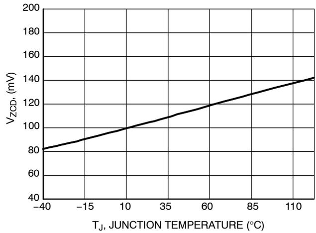
**Figure 45. Pin 6 Comparator Threshold vs. Temperature**
