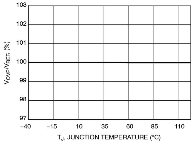
**Figure 5. Ratio Overvoltage Threshold Overvoltage Reference vs. Temperature**
