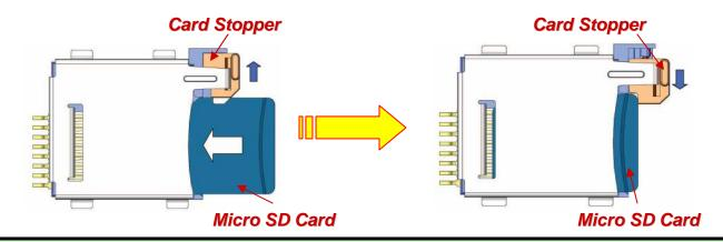
During insertion process, micro SD card pushes aside the self-retractable card stopper. Once micro SD card is fully inserted, the card stopper will return to original position by internal spring action and lock the micro SD card into position for secured connection.
