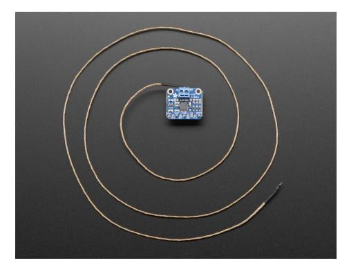
Open up File->Examples->Adafruit\_MAX31856->max31856 and upload to your Arduino wired up to the sensor. Adjust the max.setThermocoupleType(MAX31856\_TCTYPE\_K) line if necessary.
