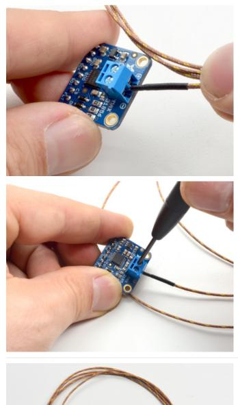
Insert the thermocouple wires and tighten down the clamps with a small Phillips or flat screwdriver
