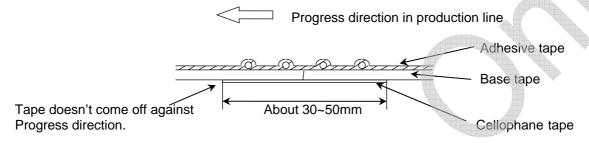
Base tape shall be spliced by cellophane tape Total tape thickness shall be less than 1.05mm
