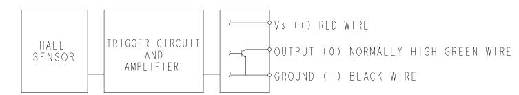
BLOCK DIAGRAM SHOWING CURRENT SINKING OUTPUTS
