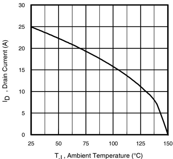
**Fig 9.** Maximum Drain Current Vs. Ambient Temperature
