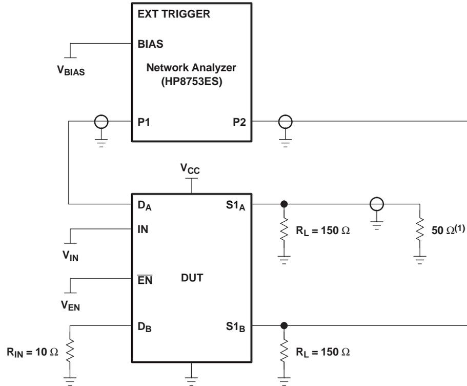
(1) A 50-Ω termination resistor is needed for the network analyzer.
