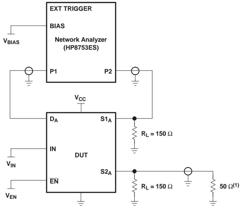
(1) A 50-Ω termination resistor is needed for the network analyzer.
