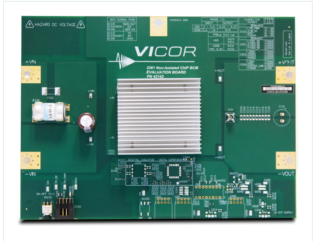
Figure 2. PCB#42142 evaluation board photo, top side
