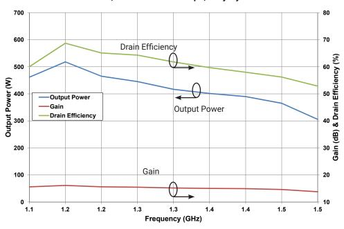
Figure 4. - CGHV14500 Typical CW RF Results  $V_{DD}$  = 50 V,  $I_{DQ}$  = 500 mA,  $P_{IN}$  = 40 dBm, Tcase = 50°C
