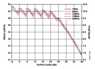
Figure 6. SINAD/ENOB vs. RxPGA Gain and Frequency
