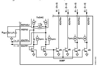
Figure 62. Equivalent Schematic of TxDAC and IAMP
