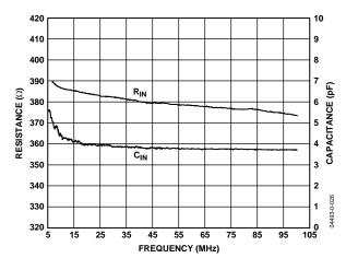
Figure 26. Rx Input Impedance vs. Frequency
