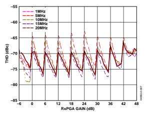
Figure 7. THD vs. RxPGA Gain and Frequency
