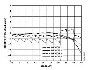
Figure 17. Rx DC Offset vs. RxPGA Gain
