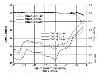
Figure 5. SINAD and THD vs. Input Amplitude and Supply  $(f_{IN} = 8 \text{ MHz}, \text{LPF } f_{-3 \text{ dB}} = 26 \text{ MHz}; \text{Rx PGA} = 0 \text{ dB})$
