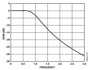
Figure 70. LPF's Normalized Wideband Gain Response
