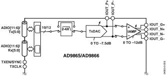
Figure 59. Functional Block Diagram of Tx Path
