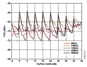
Figure 13. THD vs. RxPGA Gain and Frequency
