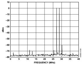
Figure 30. Dual-Tone Spectral Plot of TxDAC's Output  $(f_{DATA} = 80 \text{ MSPS}, 2 \times \text{Interpolation}, 10 \text{ dBm Peak Power}, F1 = 27.1 \text{ MHz}, F2 = 28.7 \text{ MHz})$
