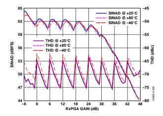
Figure 8. SINAD/THD Performance vs. RxPGA Gain and Temperature ( $f_{IN} = 5 \text{ MHz}$ )
