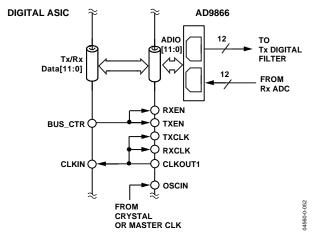
Figure 52. Example of a Half-Duplex Digital Interface with AD9866 Serving as the Master
