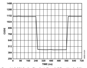
Figure 24. RxPGA Settling Time for 0 dB to +5 dB Transition for DC Input  $(f_{ADC} = 50 \text{ MSPS}, LPF \text{ Disabled})$
