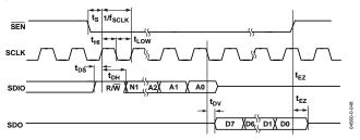
Figure 48. SPI 4-Wire Read Operation Timing
