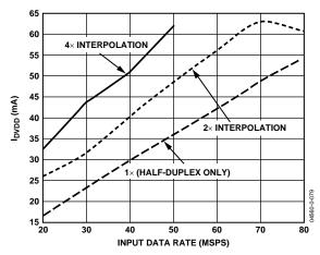
Figure 79. Digital Supply Current Consumption vs. Input Data Rate  $(DVDD = DRVDD = 3.3 \text{ V} \text{ and } f_{OUT} = f_{DATA}/10)$
