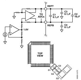
Figure 75. ADC Reference and Decoupling
