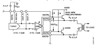
Figure 65. Voltage-Mode Operation
