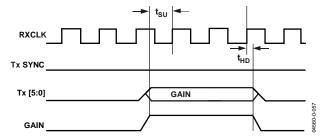
Figure 57. Updating RxPGA via Tx[5:0] in Full-Duplex Mode
