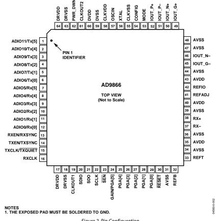
Figure 2. Pin Configuration
