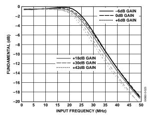
Figure 25. Rx Low-Pass Filter Amplitude Response vs. RxPGA Gain (LPF's  $f_{-3 dB} = 33 \text{ MHz}$ )
