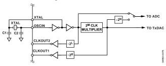
Figure 76. Clock Oscillator and Synthesizer
