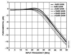
Figure 72. Effects of RxPGA Gain on LPF Frequency Response  $(f_{-3 dB} = 32 \text{ MHz} \ (@ 0 \text{ dB and } f_{ADC} = 80 \text{ MSPS})$
