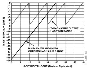
Figure 58. Digital Gain Mapping of TxPGA
