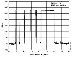
Figure 36. Spectral Plot of 111-Carrier OFDM Test Vector  $(f_{DATA} = 80 \text{ MSPS}, 2 \times \text{Interpolation})$
