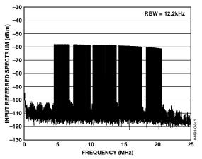
Figure 4. Spectral Plot with 4k FFT of 84-Carrier DMT Signal with PAR = 10.2 dB,  $P_{\rm IN} = -33.7$  dBm, and RxPGA = 36 dB
