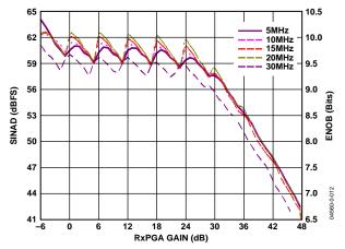
Figure 12. SINAD/ENOB vs. RxPGA Gain and Frequency
