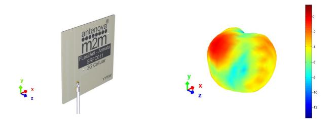
**3D pattern at 890 MHz** Drag to rotate pattern and PCB by using Adobe Reader (Click to Activate)
