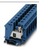
Installation terminal block, Screw connection, Cross section: 0.75 mm² - 35 mm², AWG: 18 - 2, Width: 15.2 mm, Color: blue, Mounting type: NS 35/7,5, NS 35/15
