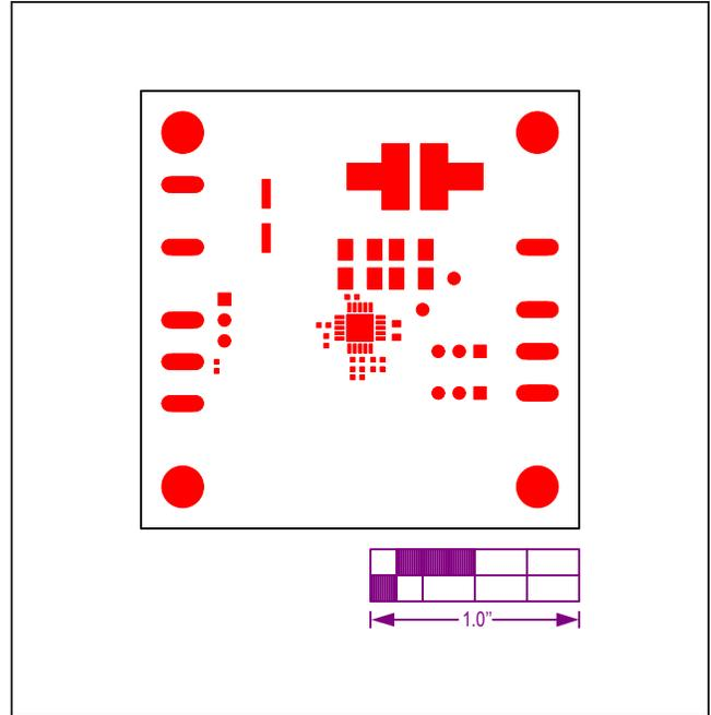
Figure 17. MAX17544 5V Output EV Kit Component Placement
