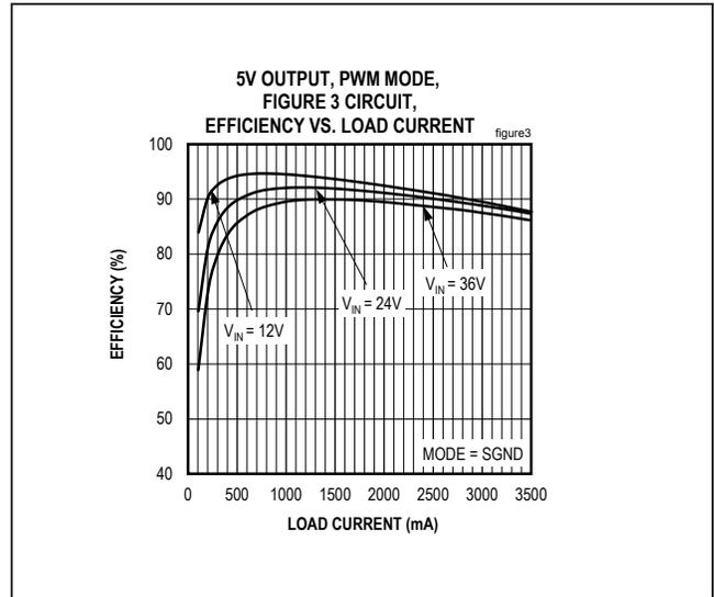
Figure 3. MAX17544 5V Output Efficiency (PWM Mode)
