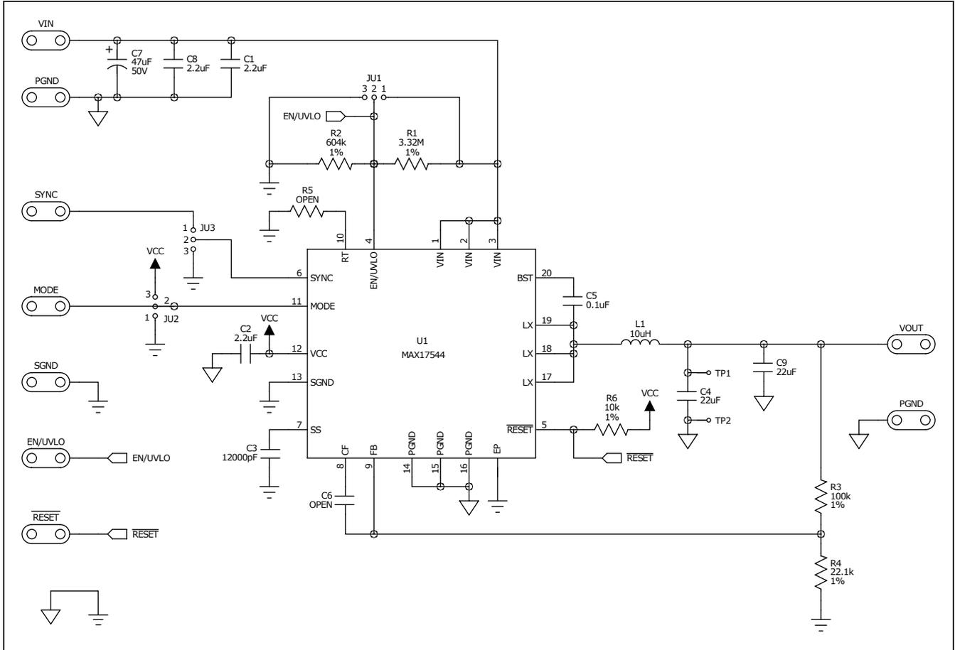
Figure 11. MAX17544 5V Output EV Kit Schematic
