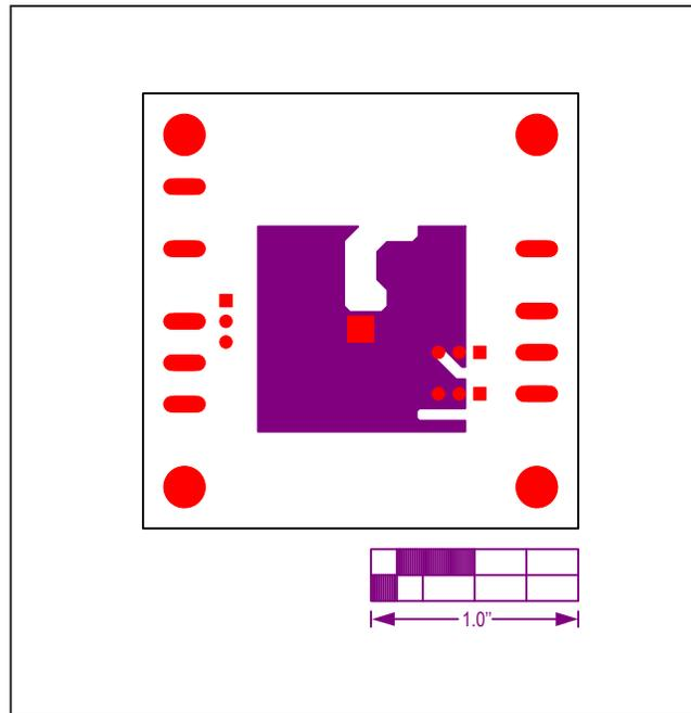
Figure 18. MAX17544 5V Output EV Kit Component Placement
