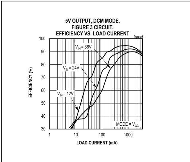
Figure 5. MAX17544 5V Output Efficiency (DCM Mode)
