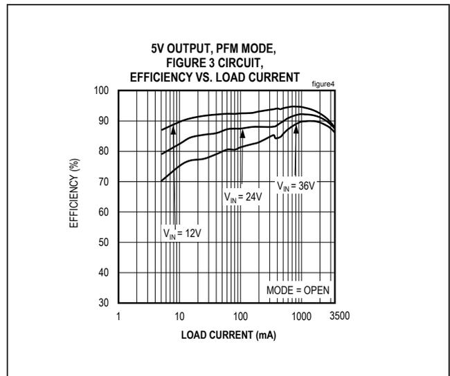
Figure 4. MAX17544 5V Output Efficiency (PFM Mode)
