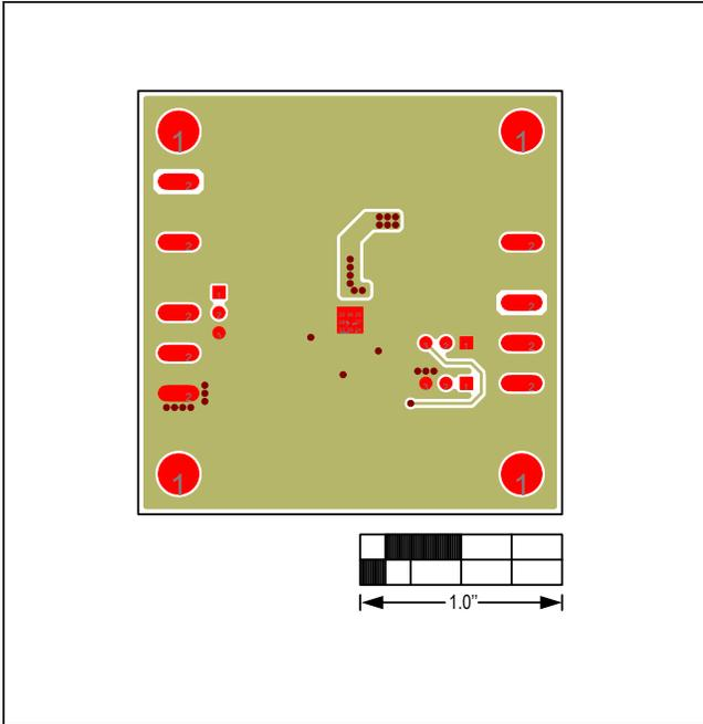
Figure 16. MAX17544 5V Output EV Kit PCB Layout—
