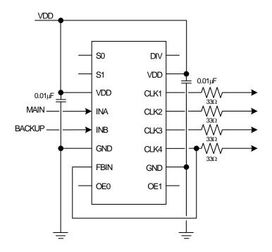
In this example, the clocks are 155 MHz and so the frequency range is address 11. Both S0 and S1 are left unconnected, causing the on-chip pull-ups to produce the required high inputs. The same is true for OE0, OE1, and DIV. In this example, CLK4 is used as the feedback. Note that the feedback path is before the series resistor.
