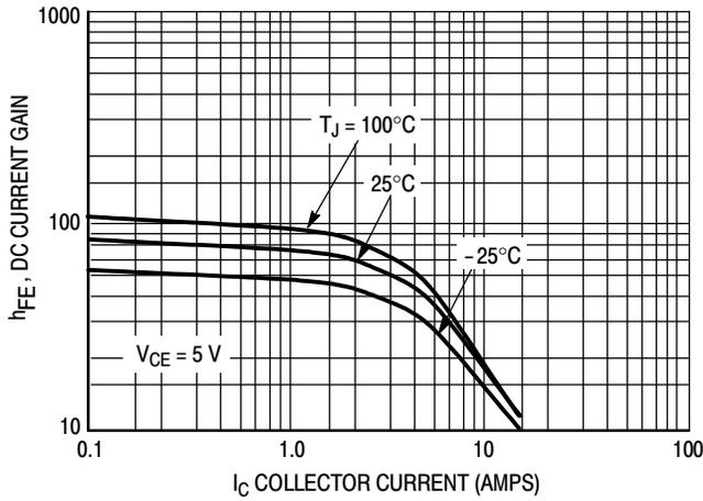
**Figure 5. DC Current Gain,  $V_{CE} = 5\text{ V}$**
