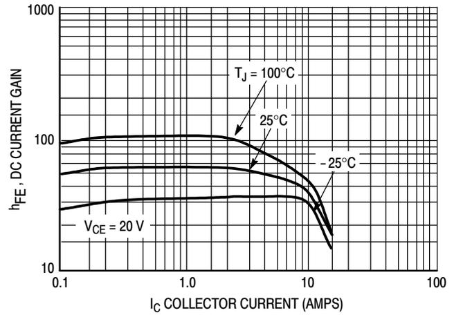
**Figure 6. DC Current Gain,  $V_{CE} = 5\text{ V}$**
