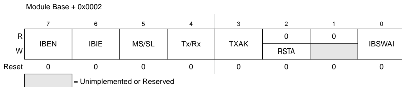
Figure 12-6. IIC Bus Control Register (IBCR)
