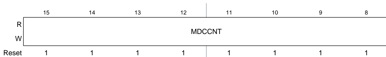
Figure 21-6. Modulus Down-Counter Count Register High (MDCCNT)
