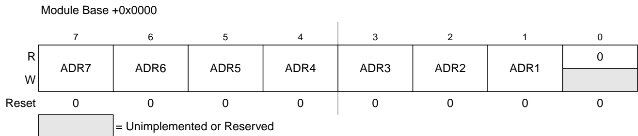
Figure 12-3. IIC Bus Address Register (IBAD)
