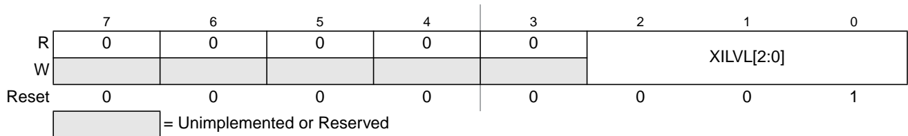
Figure 4-4. XGATE Interrupt Priority Configuration Register (INT_XGPRI0)
