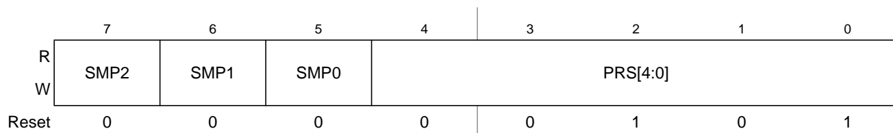
Figure 10-7. ATD Control Register 4 (ATDCTL4)
