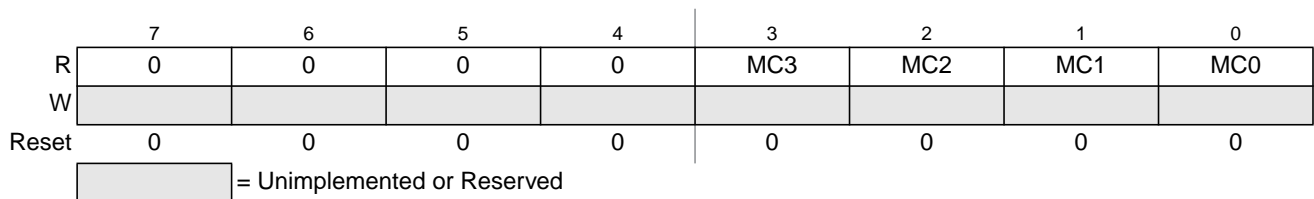
Figure 6-12. Debug Match Flag Register (DBGMFR)
