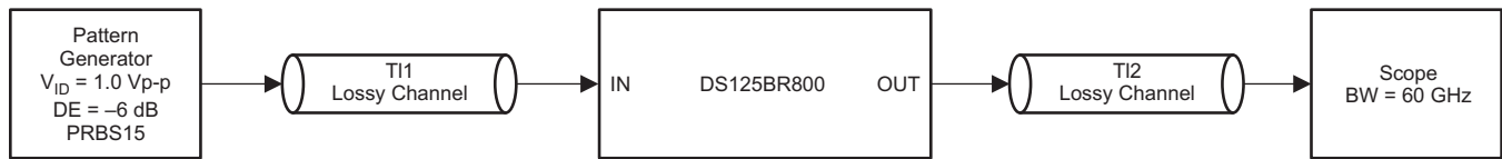
Figure 11. Test Setup Connections Diagram
