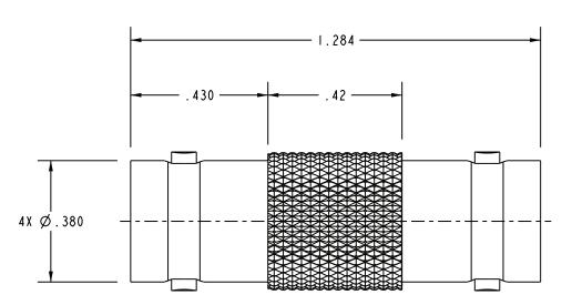
2. WITHIN SERIES FEMALE BNC FEEDTHRU ADAPTER,  $50\Omega$  AND  $75\Omega$  VERSIONS
