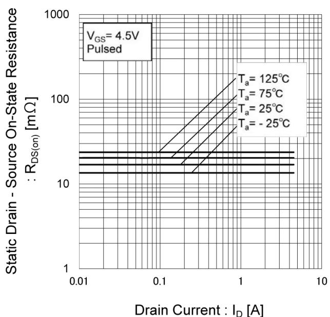
Fig.16 Static Drain - Source On - State
