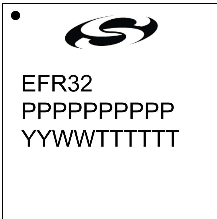
Figure 8.3. QFN48 Package Marking
