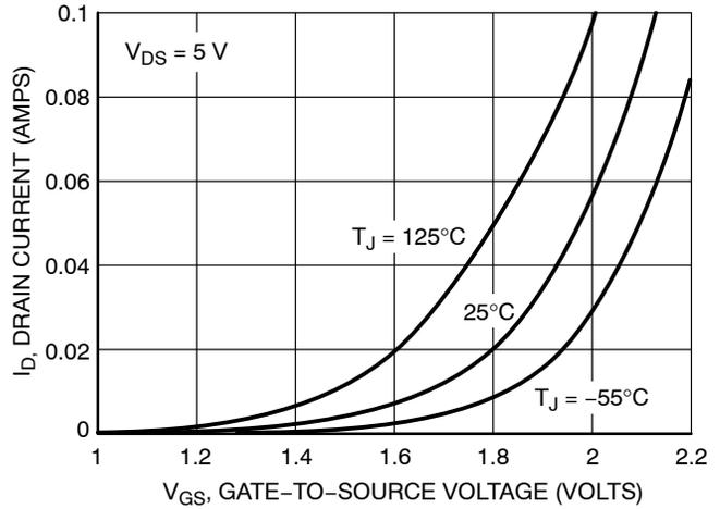
Figure 2. Transfer Characteristics
