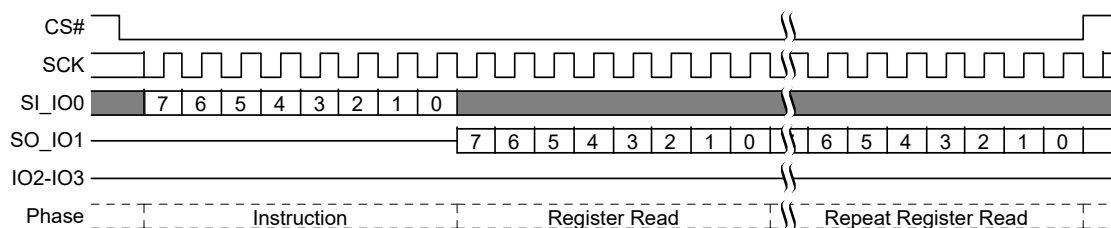
Figure 56. Read Configuration Register (RDCR) Command Sequence
