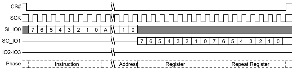
Figure 110. PPB Read Command Sequence
