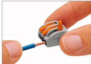
**2.** Open clamping unit using
