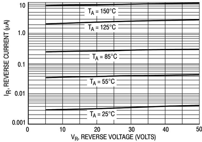
Figure 2. Leakage Current
