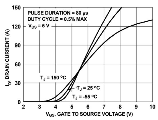
Figure 5. Transfer Characteristics
