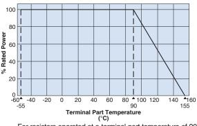
For resistors operated at a terminal part temperature of 90°C or above, the power rating shall be derated in accordance with the above derating curve.
