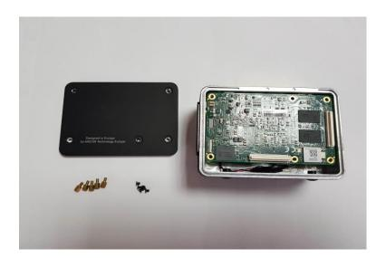
2. Fasten the UPCP PCB on top cover by 2 different kinds of hex standoffs through the 5 threads nut on (picture below). Make sure to place the 4 pcs 9mm and the 19.5mm hex standoffs in the same position as following picture.
