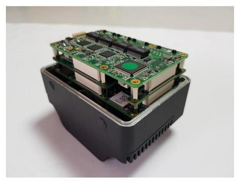
5. Place the NET Plus housing on the top of the main housing, checking the IO side, make sure the I/O is exactly matching the panel side.
